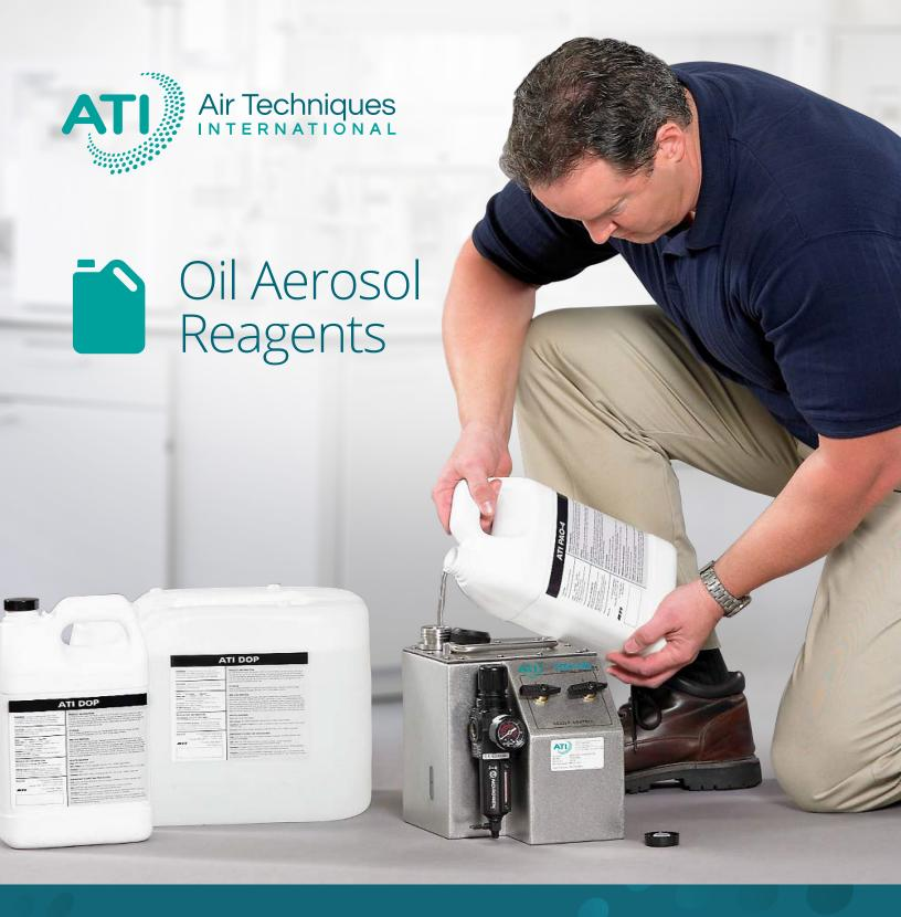
ATI offers the highest quality, industry-standard oil reagents for use in conjunction with oil aerosol generators. Our reagents are used for in situ leakage testing and production quality control efficiency testing of high efficiency air filters. ATI oil aerosol reagent products are suitable for government, nuclear, and FDA-regulated testing applications.
